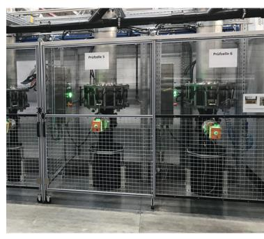
To ensure the high quality standard, the butterfly valves are tested under the toughest conditions in a test stand.
