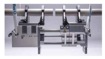
The SP 63 Mobile is available for dimensions with OD 20 mm (1/2") to OD 63 mm (2").
