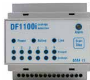
Monitoring-and location system DF1100i for 6 sensors; selective monitoring
