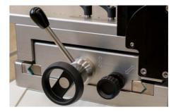
Parallel guided height and lateral adjustment of the clamping jaws for exact tension-free alignment of the welding zone with minimal pipe misalignment.
