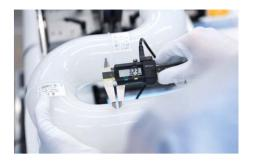
All welding parameters predefined by AGRU, such as temperature, joining pressure and welding times, are constantly monitored, controlled logged and regulated depending on ambient temperature, which is also constantly measured. QA/QC guidelines for evaluating welds and precise bead measurement by an integrated calliper guarantee excellent and reliable weld guality for each material.
