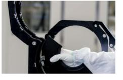
Magnetic clamping inserts enable a fast, easy and particle-free changing to other dimensions without any additional tools.
