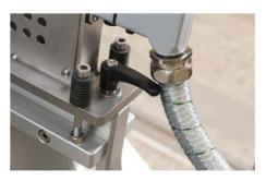
The heating element can be firmly locked with a clamping lever for safe transport.
