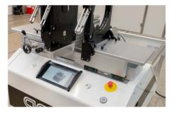
Longer external tables for the main clamping jaws facilitate the clamping of large parts, such as0 diaphragm valves.
