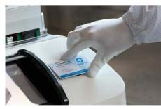
RFID data input for system access and welder identification in combination with the pre-programmed welding processes ensure a very safe and automatic welding process.
