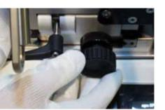
Mechanical vertical and horizontal adjustment of the clamps for precise, tension-free alignment of the welding zone and lowest offset.
