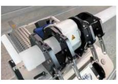
The newly designed planer and heating element are arranged in a way which ensures full 360° visibility and access to the welding area for complex isometrics.
