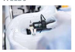
All welding parameters predefined by AGRU, such as temperature, joining pressure and welding times, are constantly monitored, controlled logged and regulated depending on ambient temperature, which is also constantly measured. QA/QC guidelines for evaluating welds and precise bead measurement by an integrated calliper guarantee excellent and reliable weld quality for each material.
