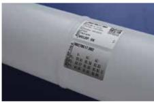
"Ongoing job report" on the machine, QR code and mobile AGRU app record all welding parameters, such as temperature, joining pressure and time.
