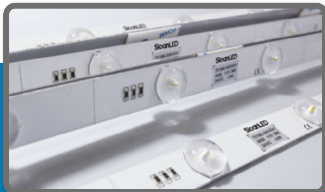
Micro prism lens producing a wide, even light spread
