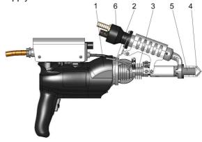
Type **MAK** is a hand extruder with integrated air supply (Autoair).
