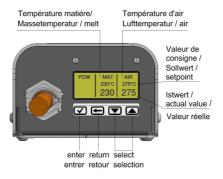
The melt temperature must have reached the preset start interlock temperature for the startup timer to be activated. After the startup timer has timed out, the start interlock will be released and the extruder can be started.
