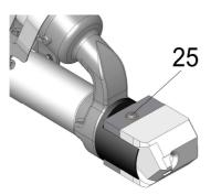
Care must be taken to ensure that the preheat nozzle provides intensive and uniform preheating (melting) of the base material over the entire joint width at as low a hot air temperature as possible. For larger weld seam widths, a wider preheat nozzle is available as an accessory.
