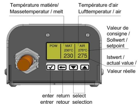
**Operating Instructions MUNSCH-controller (MA/EK-18-32) from Software 1v56 onwards
